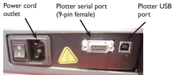
Figure 6. Locations of the power cord outlet, serial port and USB port on the rear panel of the cutter.
