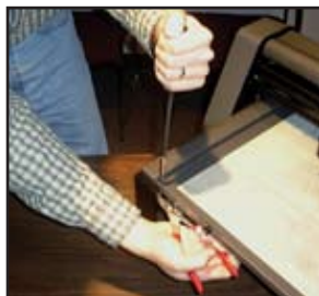
Figure 2. (Left) remove the shipping screws from the Table and (right) cut the shipping tie wrap holding the carriage .
